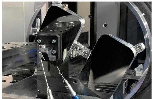
Fig. 2: Diamond turning of two aluminum mirrors.
