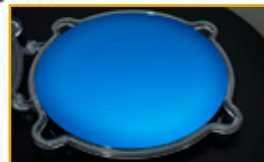
300 mm silicon wafer with BaTiO 3 .
